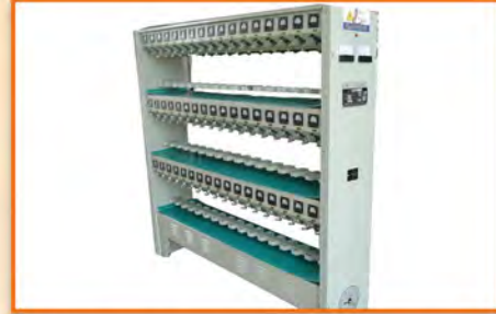
Miner's Lamp Charging Rack
